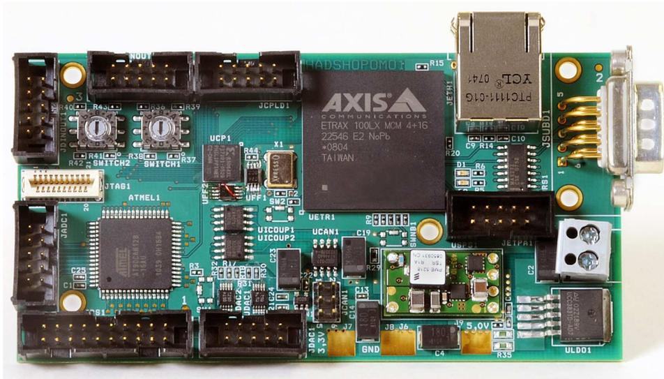
Abbildung 11.4: HADES Control general purpose board, HadCon [Zum12]
