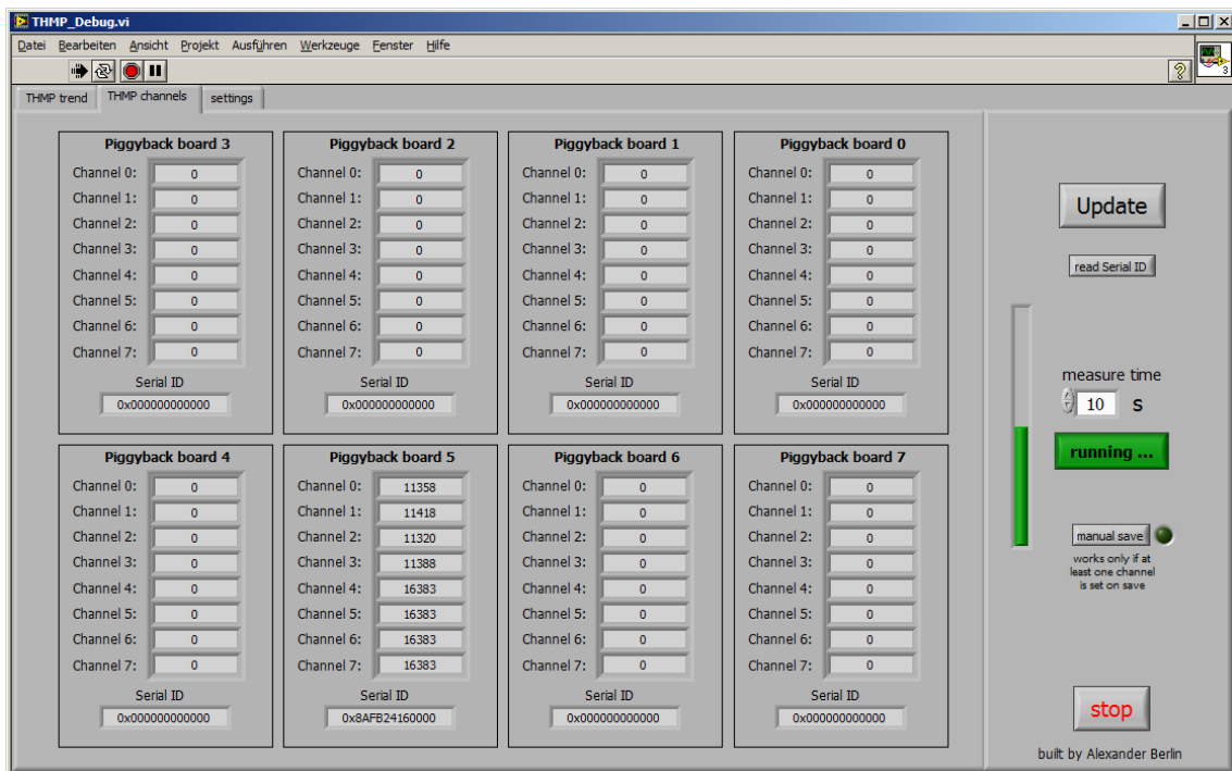
Fig. C.2 – Channel window of the THMP LabView program. This window presents an overview of all sensors, ordered for each module.
