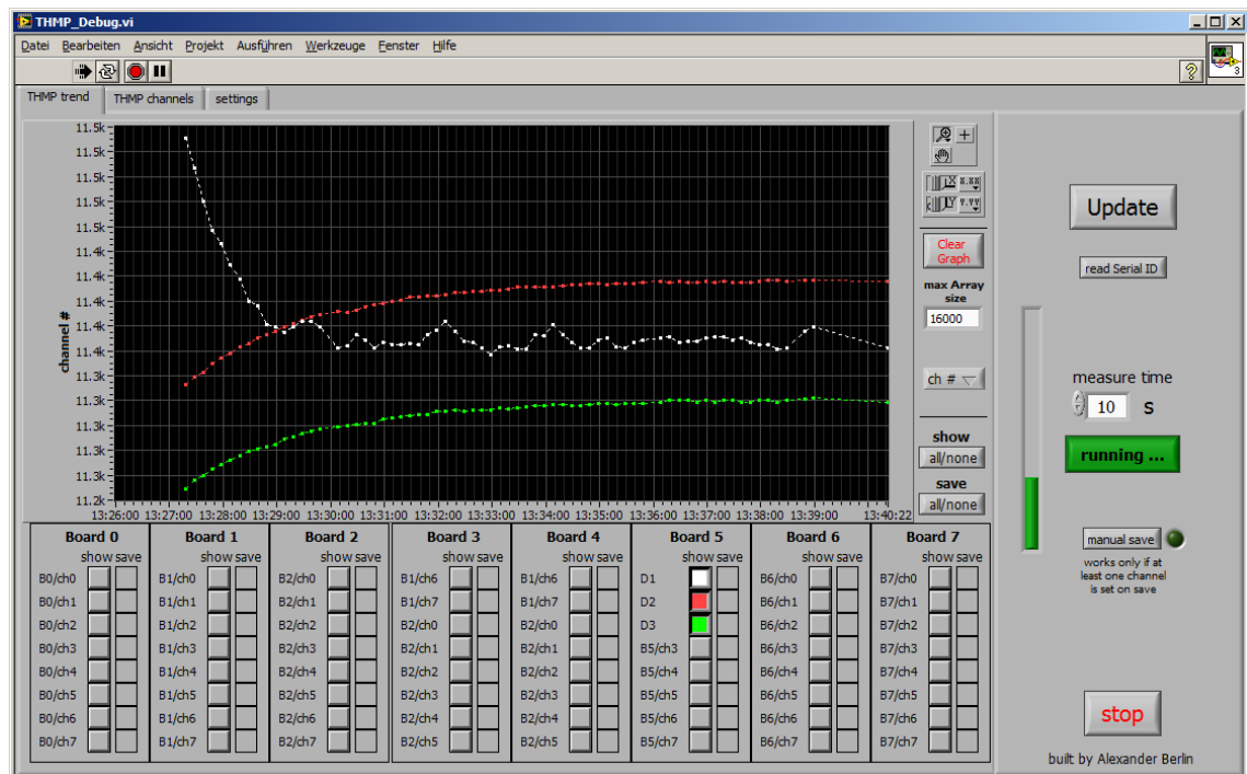
Fig. C.1 — Trend window of the THMP \overline{\text{P}} LabView program. All possible 64 sensors can be displayed, selected and/or stored. Also the graph can be switched from channels to voltages.
