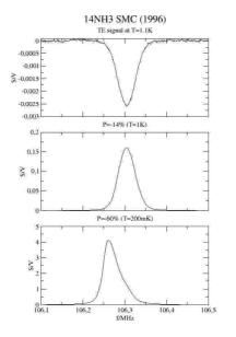
TE - Signal - T = 1.1 K - B = 2.5 T  $^{4}$ He - cryostat - T = 1 K - B = 2.5 T - P = -14 % Dilution - cryostat - T = 200 mK
