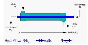
At low temperatures, the main impediment to heat transfer is the thermal boundary (Kapitza) resistance  $R_k$  between the helium and the HX walls
